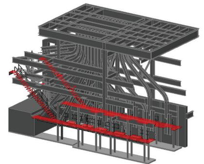
Lockett & Farley used Revit to highlight projected demolition. Image courtesy of Lockett & Farley.
