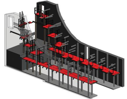
Lockett & Farley used Revit to highlight new maintenance platforms. Image courtesy of Lockett & Farley.
