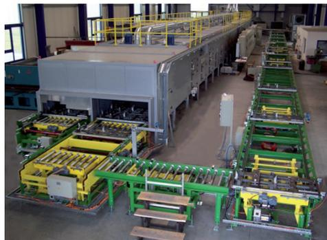
Drying system for molds of car engine blocks (Image: ELPO GmbH).
