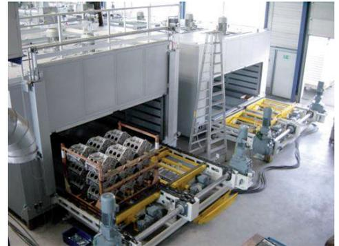
Heat-treatment system for car engine blocks (Image: ELPO GmbH).
