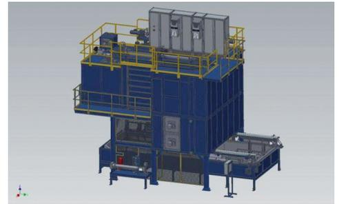
System to chill and dry safety-relevant car body parts (Image: ELPO GmbH).
