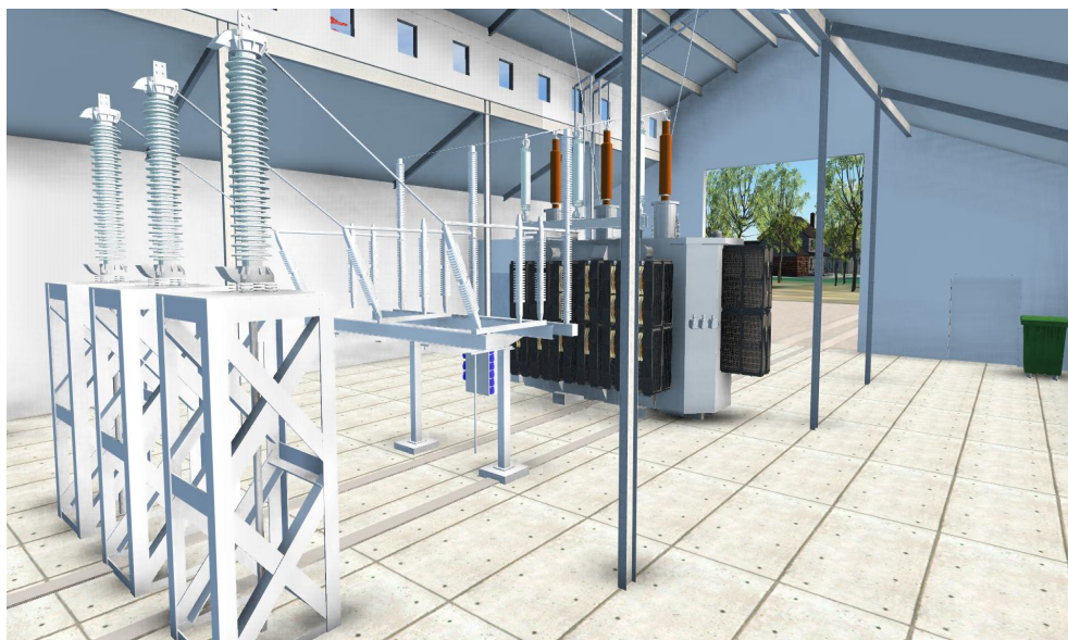
Conceptual design for an indoor substation in Autodesk InfraWorks 360. Image courtesy of Idaho Power.
