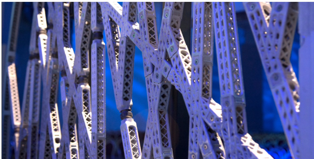
Airbus bionic partition. Image courtesy of APWORKS
