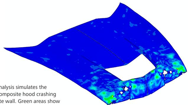
Composite Analysis simulates the effects of a composite hood crashing into a concrete wall. Green areas show matrix or intermediate damage, white holes show material loss (i.e., element deletion) due to fiber damage.
